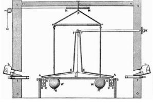
A cut away view of Cavendish's apparatus set in its closed chamber with observations being performed from outside.
