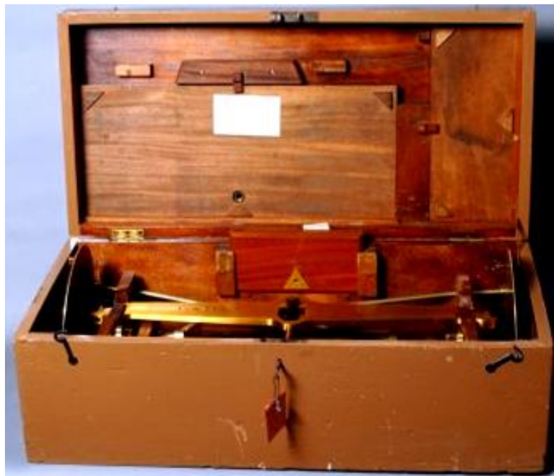
An example of a 56lb 'outdoor' inspector's beam, preserved in a UK collection. It could be easily packed away into its carrying box and taken to the coal-yard. 56lb weights were checked to an accuracy of 50 grains (just over 3g)
